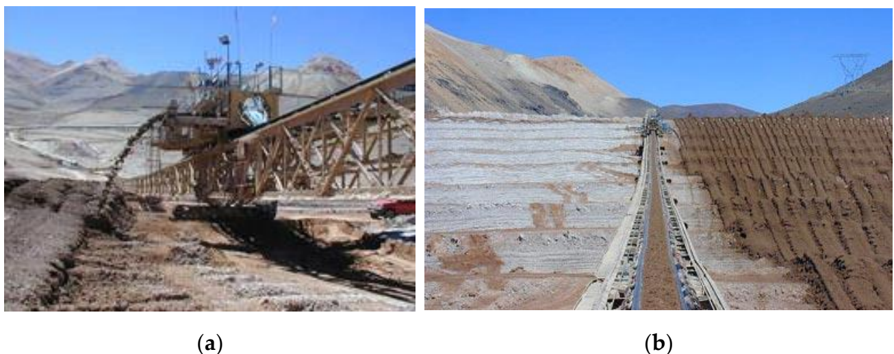
Figure 21. Dry stacking of filtered tailings at La Coipa, Atacama region, northern Chile, showing (a) stacker, and (b) overall stack [29].
