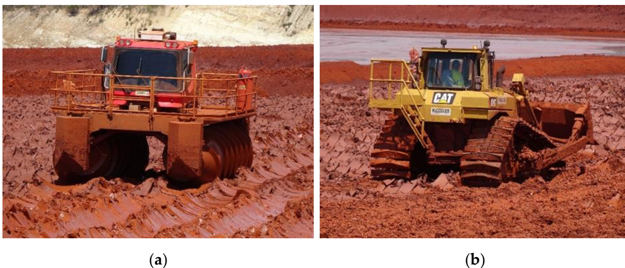
Figure 19. Farming red mud, by (a) a scroller, and (b) bulldozing with a D6 Swamp Dozer.
