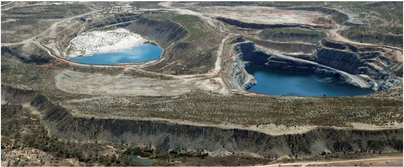
Figure 23. In-pit co-deposition of waste rock and thickened tailings (left-hand pit) at Kidston Gold Mines in north Queensland, Australia.
